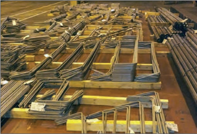
△ Stainless steel reinforcement having been fully cut and bent at Outokumpu's Sheffield Stainless Bar facility for the new Allt Chonoglais bridge
